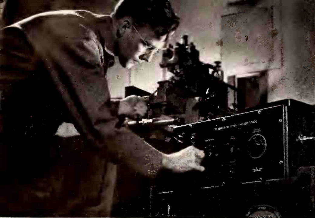
Radio tubes are used in this Chronoscope to measure bullet speeds in milliseconds.
